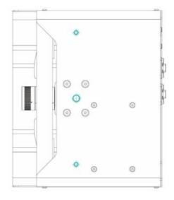
▲The bottom plate of the 2000 Series – 1/4" UNC in the middle and M6 screw holes
